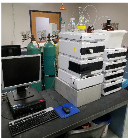
Figure 4a. A high-pressure liquid chromatography (HPLC) machine used to analyze cannabinoids in hemp.
