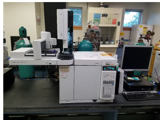
Figure 3. A gas chromatograph that is used to analyze volatile compounds.
